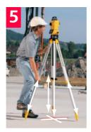
Adjust the legs of the tripod to level the circular level
