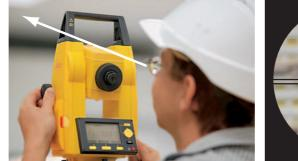
Target Point roughly using the notch.
