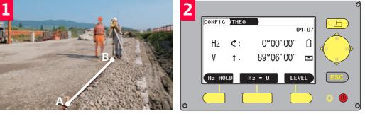
Setup and level the instrument over point B.
