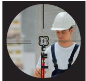
Using the telescope, overlay crosshair and prism center.
