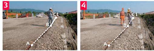
Flip the telescope (i.e. reverse it) and mark Turn the instrument 180°(200 gon) and point C1.
