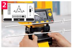
Center the electronic level of this axis by turning the two footscrews. Arrows show the direction for rotating the footscrews.
