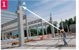
Setup and level the instrument. Target high point A
