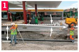
Setup and level the instrument on a point along the straight line the slope of which is to be determined. Position a staff at a second point along that line.
