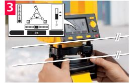
When the electronic level is centered the arrows are replaced by checkmarks.
