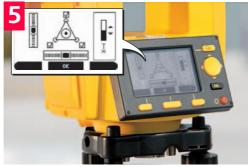
When the electronic level is centered and three checkmarks are shown, the instrument has been perfectly leveled up. Accept with OK.
