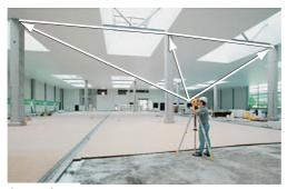
Polygonal With Polygonal method, the tie distance is With Radial method, the tie distance is always computed between subsequent points. If all distances should be measured from the same startpoint always, then chose the radial method below:
