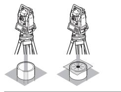
Under some circumstances the laser dot is not visible, for example over pipes. In this case, the laser dot can be made visible by using a transparent plate so that the laser dot can be easily aligned to the center of the pipe.
