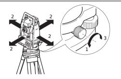
If the instrument is equipped with the optional shifting tribrach it can be aligned to the ground point by slight shifting.
