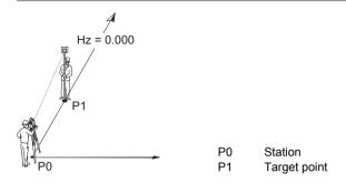
Setup method Establish Control Line -Over 1<sup>st</sup> Point stepby-step
