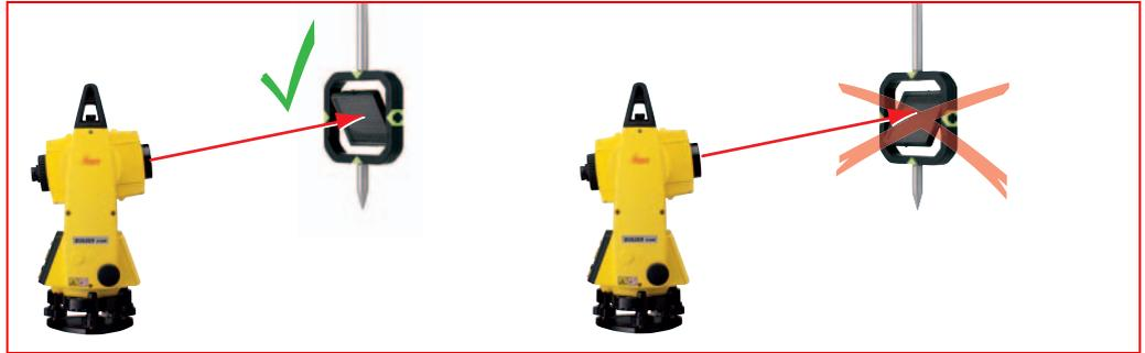
Tilt the moving part of the flat prism correctly.
