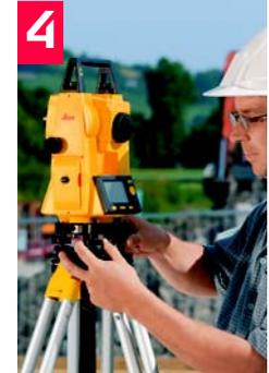
Use the foot screws of the tribrach to centre the plummet on the ground point. Ignore that the instrument is not yet levelled precisely.
