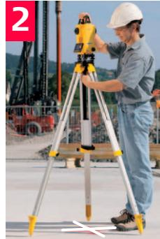
Fasten the tribrach and the instrument on to the tripod.
