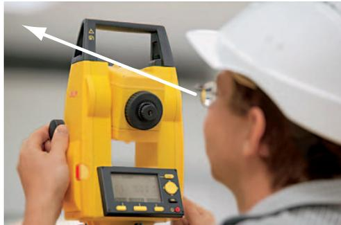
Target Point roughly using the notch.
