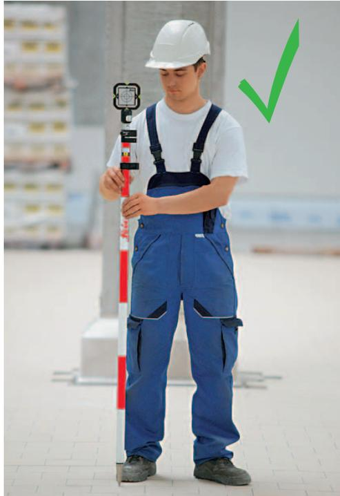
Holding the reflector pole correctly
